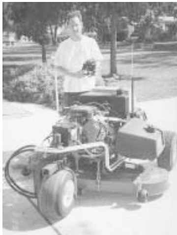
"It turns a lot of heads when people drive by my front yard and see me operating it from my driveway," says Jeff Parker about his home-built, radio-controlled mower.
