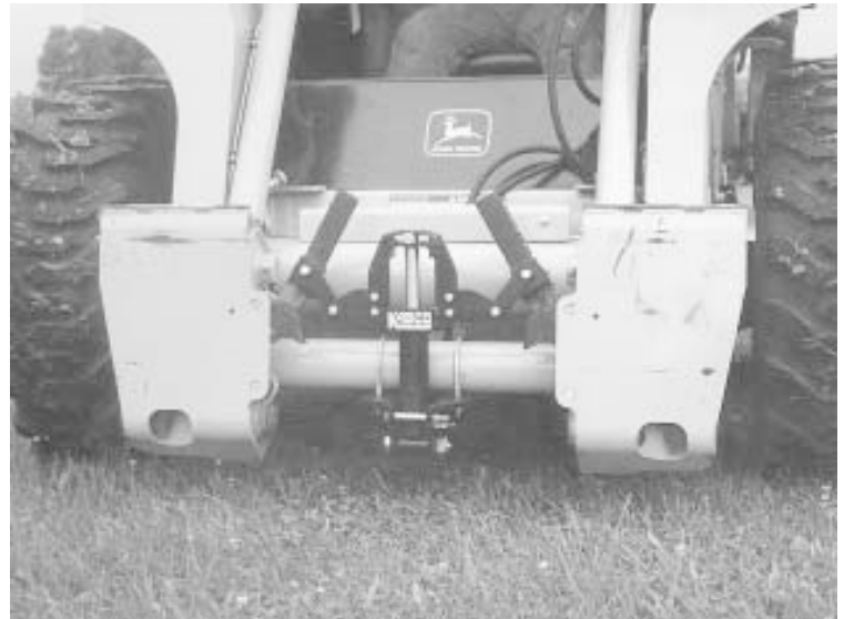
Hydra-Hitch uses a small cylinder to hydraulically move a pair of latch pins up or down, virtually eliminating the need to ever get out of the cab, says the company.
