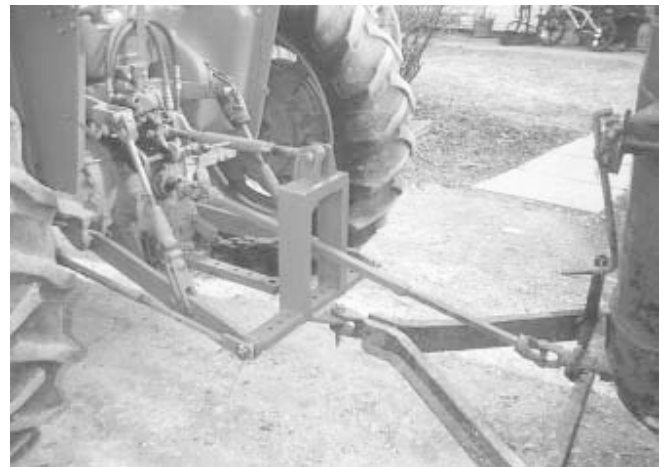
Seltzer welded an open steel frame onto his tractor drawbar. Top of frame hooks to the 3-pt. top link, which makes the drawbar rigid. A pto shaft can run through frame.
