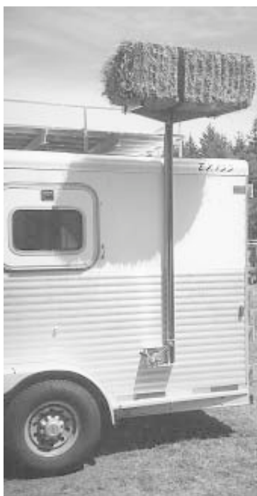
Aluminum rail attaches to outside wall of trailer. It's fitted with removable lift arms that carry bale up to roof.
