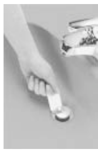
Zip-It is a 20-in. long plastic strip with barbs on either side. You stick it down into the drain and pull it back out to clean plug-ups.
