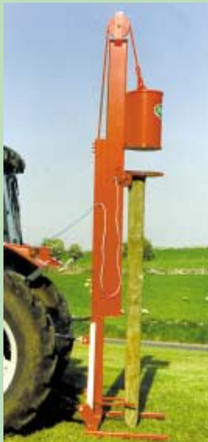
Wood post driver is equipped with an 800-lb. hammer (above). Driving plate (left) is fitted with two small spikes that grab post.
