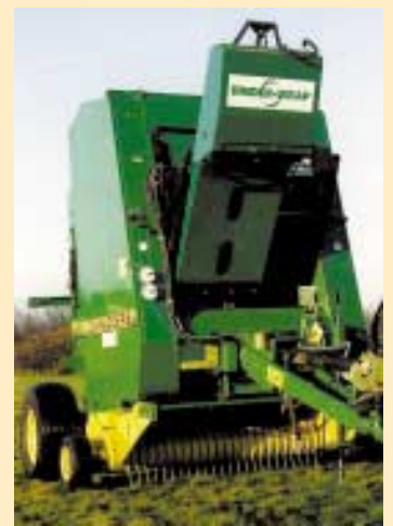
"Binder-Wrap" mounts on front of baler and holds a single roll of plastic stretch film. It lets you wrap round bales with plastic film right inside the baler, without using any twine or net wrap.
