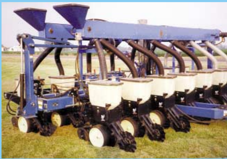
Hydraulic-operated "seed belt" distributor eliminates the need to drag seed vac hoses from seed box to seed box. There's just one fill point for each row of boxes.
