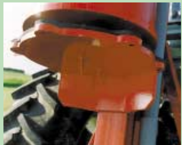
Wood post driver is equipped with an 800-lb. hammer (above). Driving plate (left) is fitted with two small spikes that grab post.
