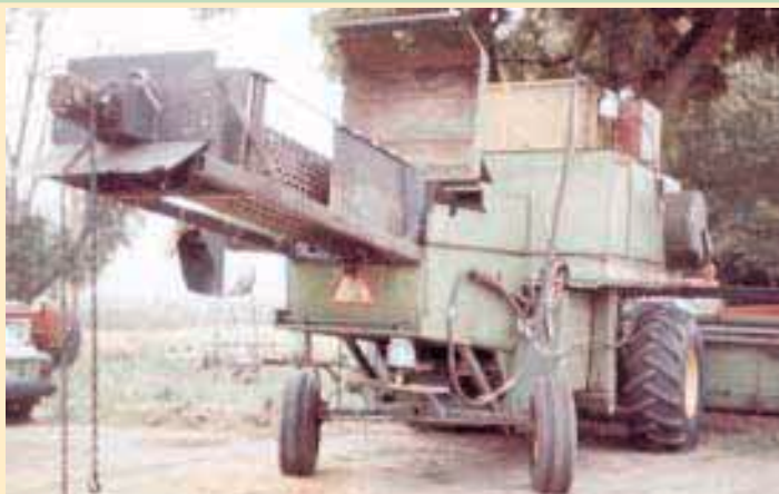
Yeager converted a conventional Deere 6600 combine to rotary by removing the straw walkers and installing his own home-built, hydraulically-powered rotary separator.
