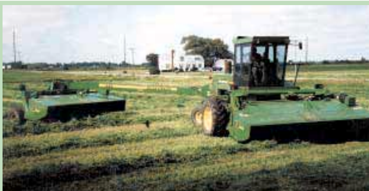
Miller converted his Deere 5460 SP chopper into a mower-conditioner by reworking the drive system to power a front mount mower and a mower that trails behind.
