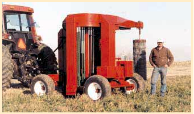
"It lets one person put up a mile of fence posts in an 8-hour workday," says inventor Tim Herrmann.
