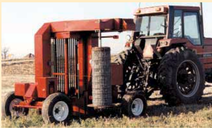
Rig is equipped with rotating "magazine" that holds supply of posts.
