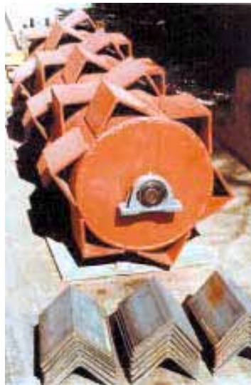
L-shaped steel brackets weld onto steel cylinder to make indentations in seedbed.
