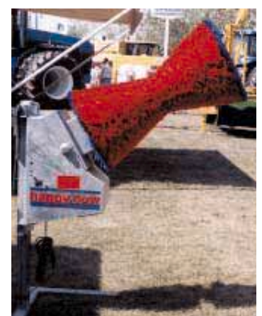
Powered rotating brush starts up automatically when a cow bumps against it. It runs for 60 seconds, then shuts off.
