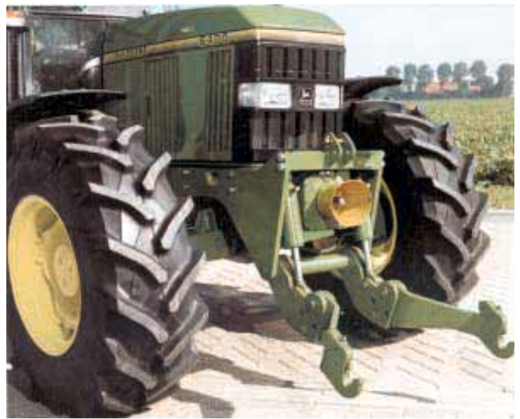
Zuidberg front 3-pt. hitch and pto is made in Holland. The company is the number one supplier of front 3-pt. hitches in Europe.
