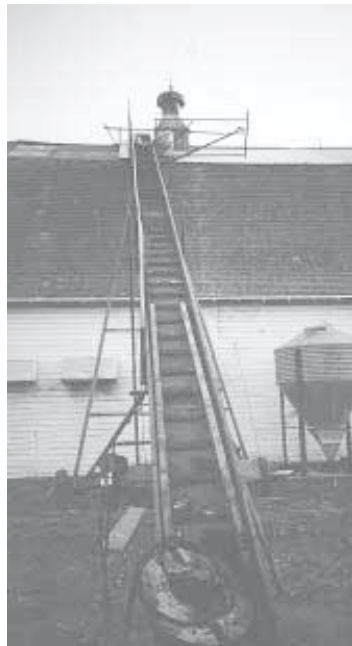
Elevator has a 12 by 4-ft. safety fence at the top, providing a safe area where Meister can sit or stand without fear of falling.
