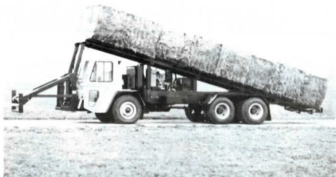
Unit consists of upfront bale fork, inclined platform over cab, and unloading endgate.
