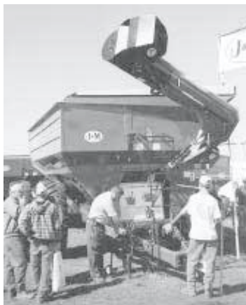
Auger mounts on front of cart where tractor driver has full visibility during unloading and fold-up.
