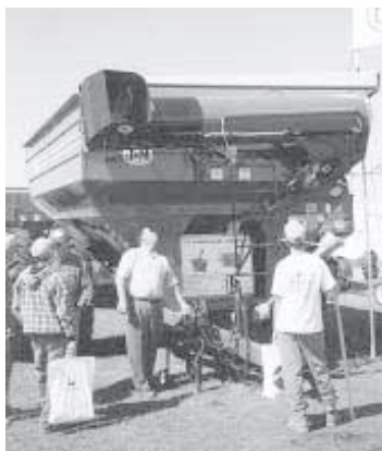
Front-folding auger takes up less space than side-unloading augers, according to J & M.
