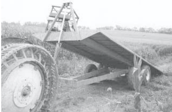
Trailer is tilted by a 4-ft. long, 4-in. dia. hydraulic cylinder attached to a steel A-frame welded at front end of trailer.
