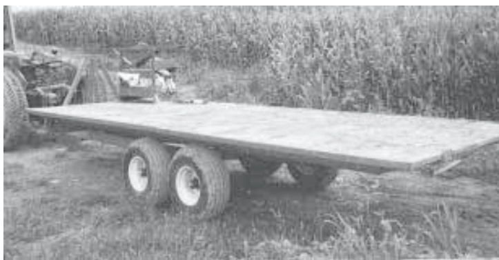
The 23-ft. long trailer uses a pair of 10-in. steel I-beams to carry the main load, with 2-in. oak planks bolted crosswise to form floor.
