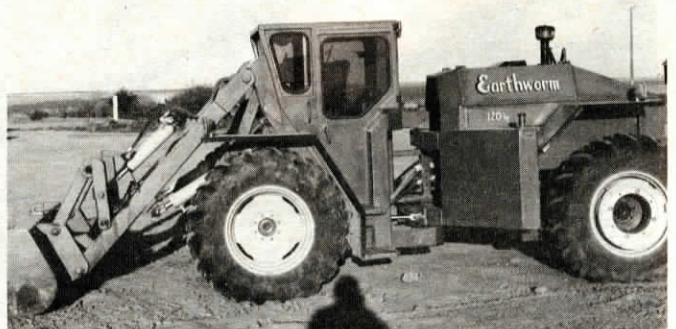
Steering wheel activates a hydraulic cylinder which bends the machine in the middle.
