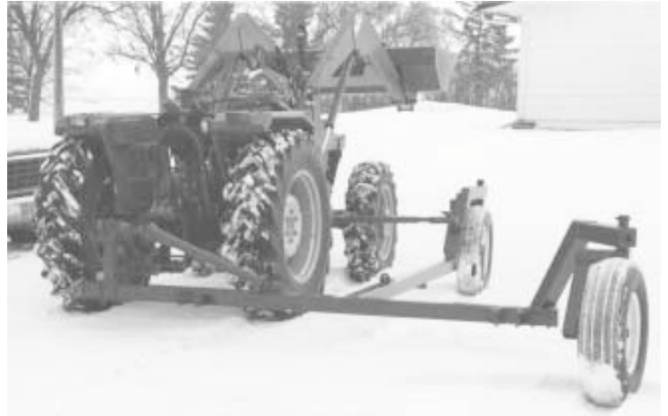
Two pivoting caster wheels allow transport frame to freely follow tractor. "Backing the auger into place is no more difficult now than backing the tractor," says Ailsby.
