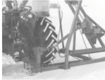
Ailsby's home-built transport frame hitches to side of tractor.
