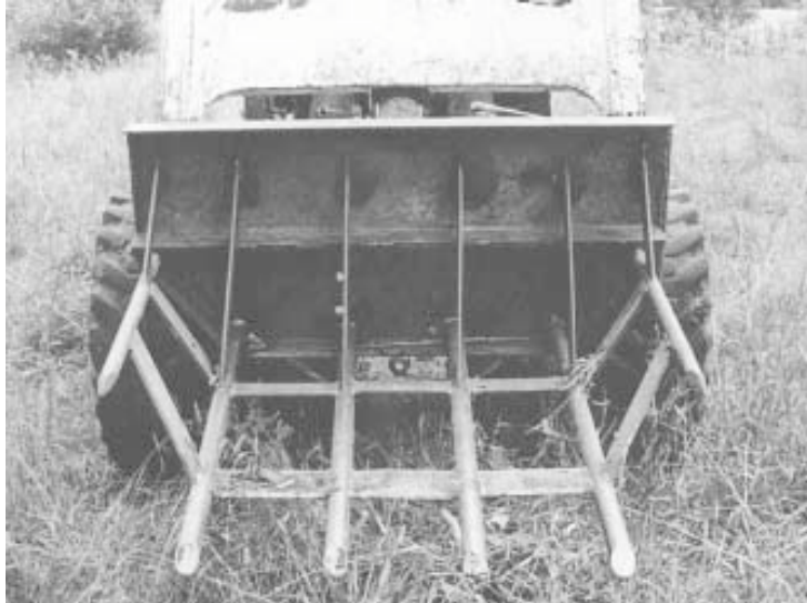
Brush fork operates just like a loader bucket, except that it doesn't disturb as much soil. To remove bushes, De Cook drives forward with shafts a few inches under ground.
