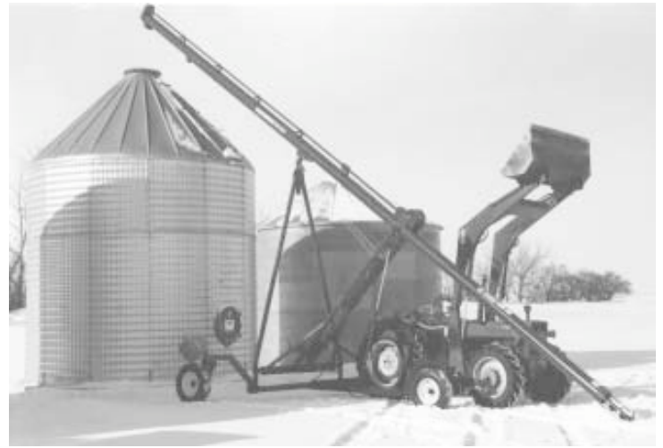
Tractor is positioned midway along auger tube so Ailsby can use auger both for filling and emptying bins. Original auger undercarriage and lift mechanisms remain in place.
