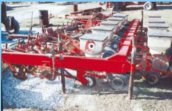
Johannes welded a U-shaped steel bracket to each side of splitter planter frame, making it possible to quickly hook up five add-on row units.
