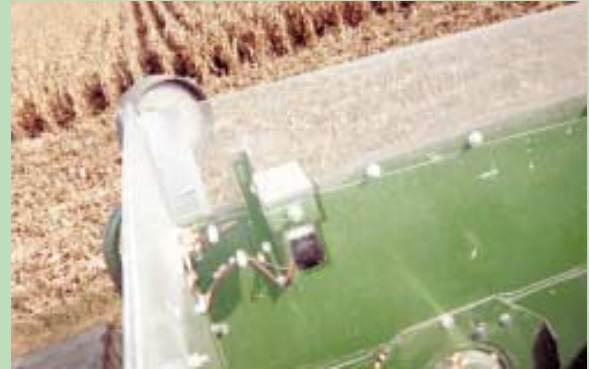
To let him know when his combine's grain tank is getting full, he installed a flapper switch about 3 in. below the top of the hopper and wired it to an alarm and flashing yellow light mounted in the cab.
