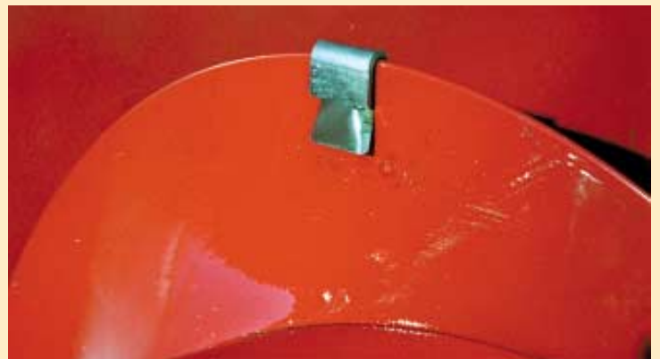
Stalk Grabbers can be quickly hammered onto flighting on feederhouse auger. They make auger more aggressive to keep crop material from piling up on corn head.
