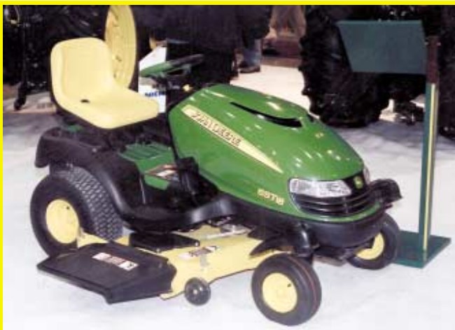
New mower uses a conventional steering wheel instead of levers to turn on a dime.
