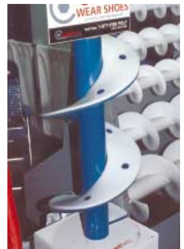
Add-on flighting comes in sections that are pre-formed and pre-drilled to fit onto either new or worn out steel auger flighting.
