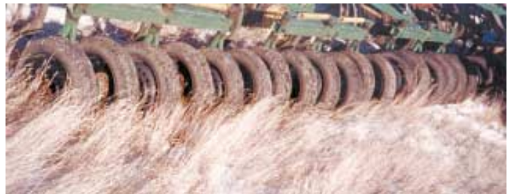
Ray and Dale Culler converted their 37-ft. Deere field cultivator into a press drill by mounting 36 "mini" spare tires on back of it.
