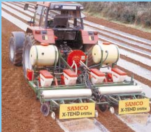
SAMCO X-Tend machine uses rollers on back to lay down plastic over row.
