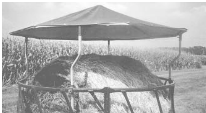
Octagon-shaped roof frame is covered by a snap-on marine-grade poly canvas and attaches with four legs to top and bottom rings of feeder.
