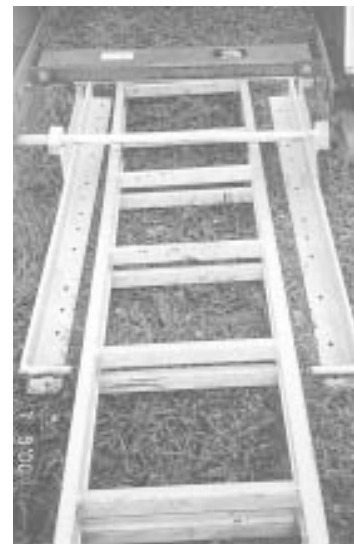
Ladder mover holds ladder in place, with legs resting on ground. Top end of ladder fitted with a pair of small wheels that roll up and down side of buildings.
