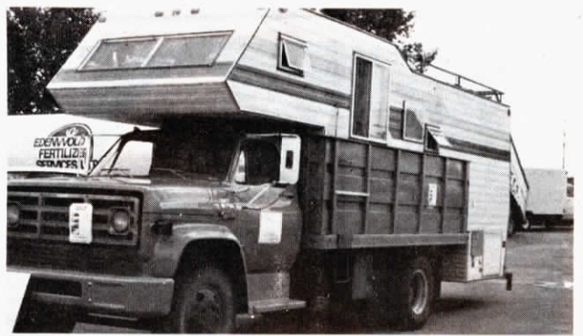
The motor home mounts on standard grain trucks and unloads without jacks or blocks.
