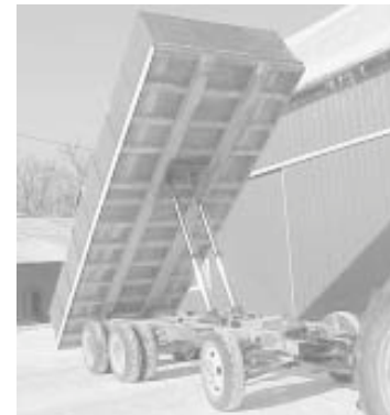
The Scotts started with the frame of an old GM bulk feed truck and built an 8 by 24 by 3-ft. deep box for it from scratch. Box is hinged at back.
