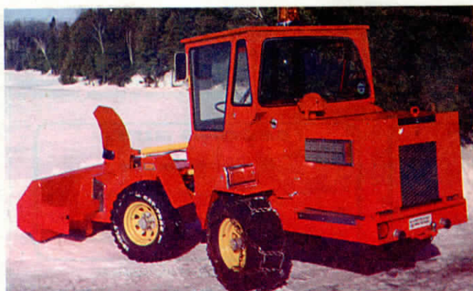
Rig's 7-ft. wide snowblower is powered by a Honda 5-speed transmission.
