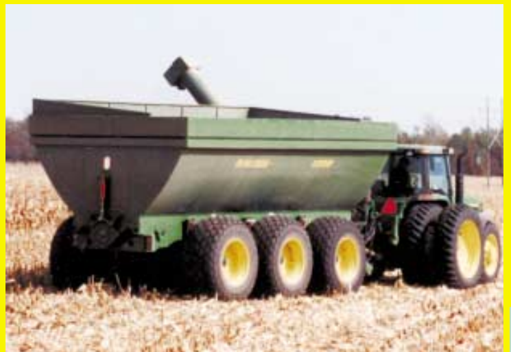
When equipped with an extension, Balzer's 6-wheel grain cart holds 1,500 bu. of corn.
