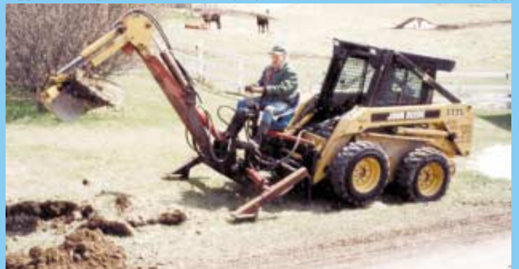
Backhoe mounts on skid loader via a 3-pt. quick hitch.
