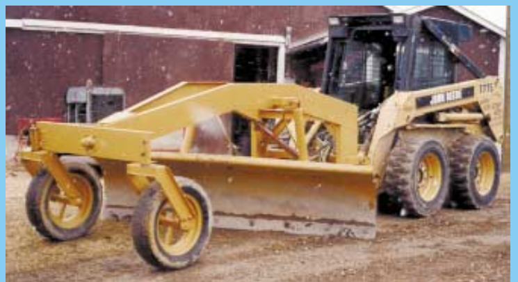
"Skid loaders do a lot of hopping and skipping, but with the frame and blade out front supported by a pair of wheels, bouncing is greatly reduced," says inventor Frank Jepp.
