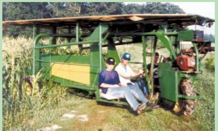
Rig is powered by a 2-cyl., 18 hp Briggs & Stratton gas engine that mounts above a single front drive wheel.
