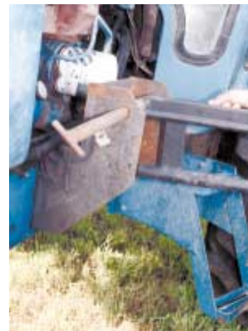
Marker arm mounts on a bracket bolted to tractor frame. For transport, a pin on each arm is pulled and the markers pivot straight up.
