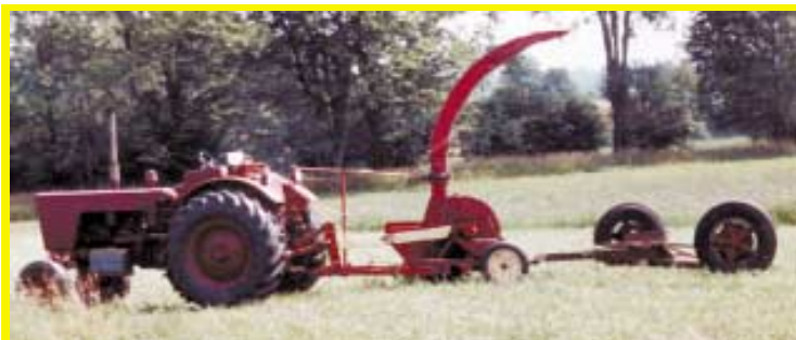
Armstrong built a towing frame using the front axle off a 4-ton truck. A cradle holds rear wheels of forage truck about 4 in. off ground.
