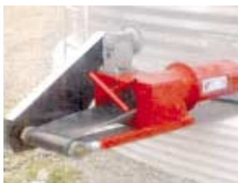
The 10-in. wide rubber belt rides inside an 8-in. steel tube, which seals tight against bin wall so it won't affect aeration fans.
