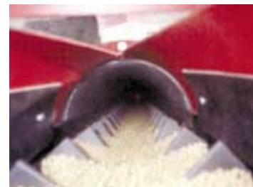
Cleats attach to flat belt that follows curvature of tube. After exiting the tube the belt flattens out again.
