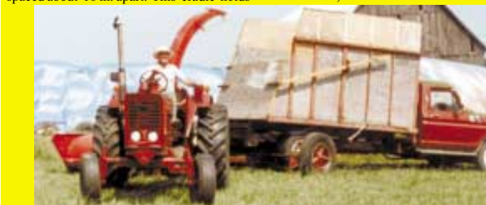
Dumping forage box mounts on back of 1-ton pickup, which he tows on cradle.
