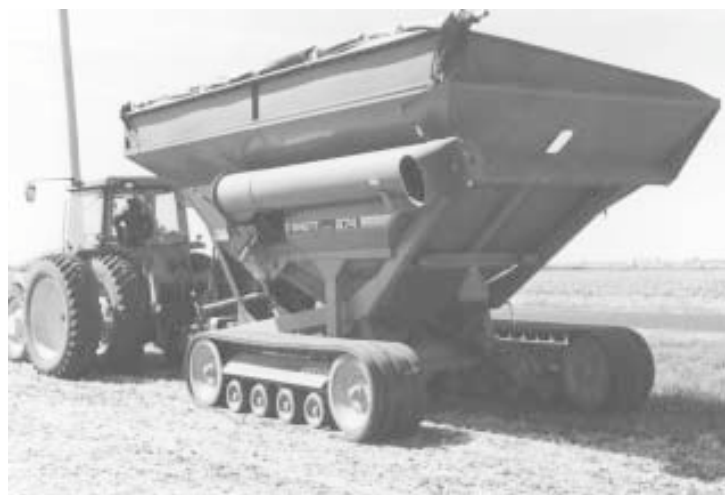
William Murphy had a local shop transfer Cat tracks from his old Kinze 800 bu. grain cart to his new 1,000-bu. Brent cart. "It saved me a lot of money," he says.
