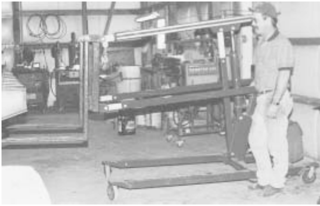
Crane is lifted by an 8-ton hydraulic bottle jack and is equipped with a pair of forks on front.
