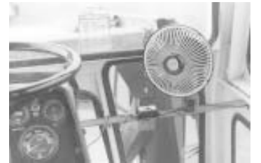
Dan Capiuk installed a $20 electric fan in his tractor cab. Fan bolts to a section of metal strap across right front corner of cab.
