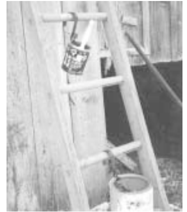
Hook bolts onto paint can and allows you to hang bucket from ladder rung.
