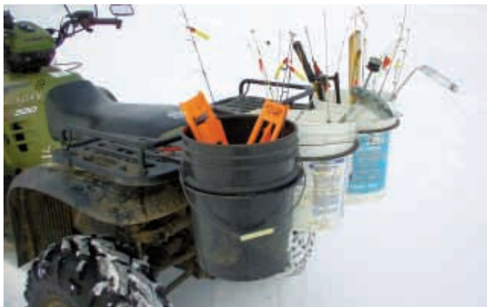
“Bucket Rack” holds three 5-gal. buckets without taking up any space on ATV’s rear rack.
