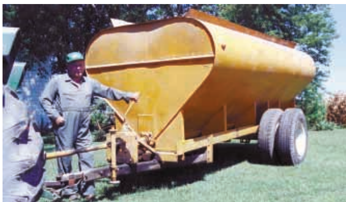
Steinacher turned a hopper from an old cement bulk trailer into this 350-bu. grain cart. A 4-speed truck transmission is used to pto-drive an auger at bottom of cart.
