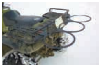
T-handled mounting bolt fits through ATV rack to hold bucket rack in place.
