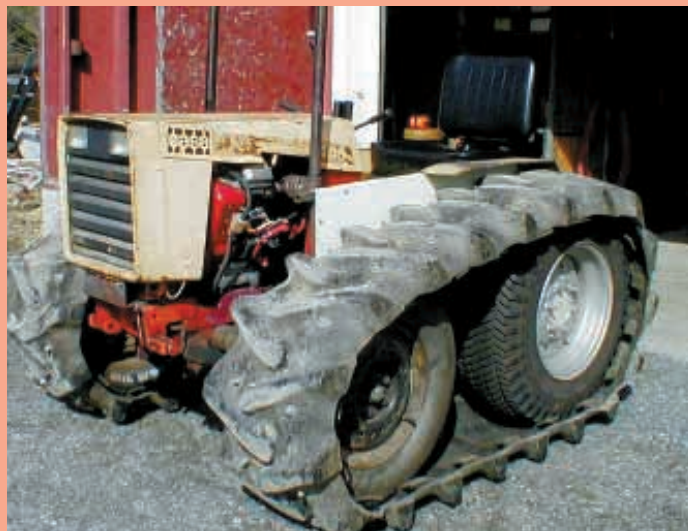
Jim Brown used the tread off a pair of tractor tires to make these tracks, which he mounted on his Case 446 garden tractor.
