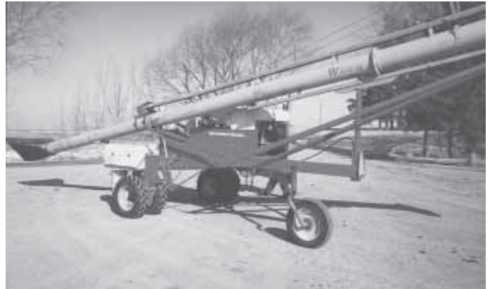
Jerry and Laurie De Blonde removed the wheels from their 44-ft. 10-in. Westfield grain auger and mounted it on an IH self-propelled swather.
