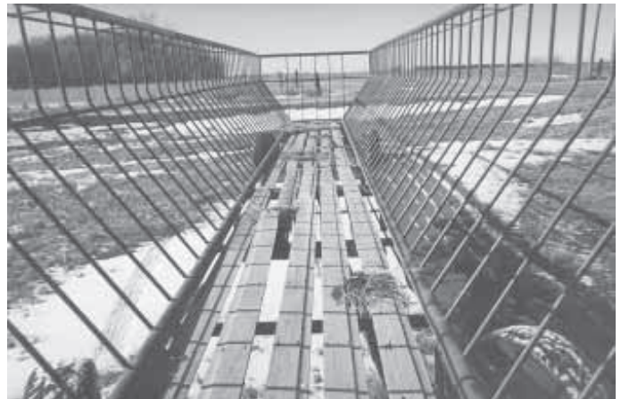
Because feeder is steerable at either end, it's easy to maneuver in and out of pastures.
