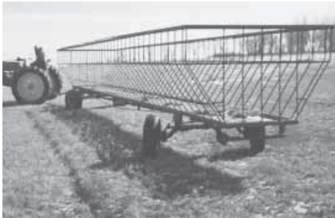
Tongue can be easily detached and re-attached at opposite end of rig.
