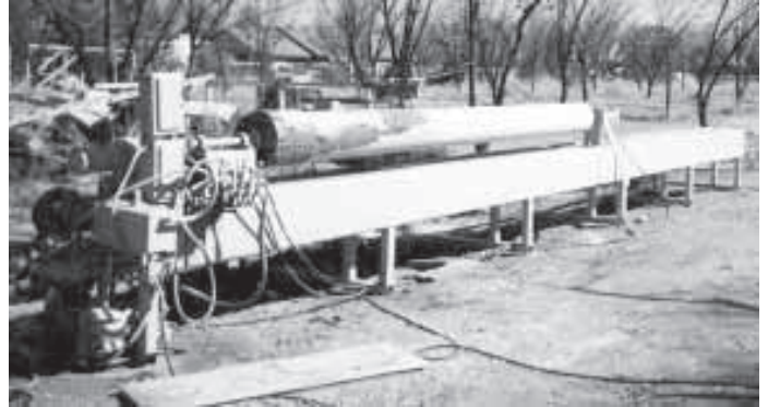
Green uses his log lathe to “turn” logs to a uniform diameter for building houses.
