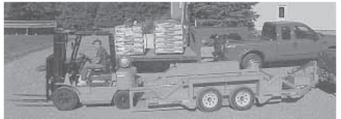
Trailer deck lowers via DC motor powered, self-contained hydraulics.
