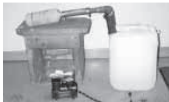
A couple of 12-volt air compressors pump air into a pair of 5-gal. plastic pails.
