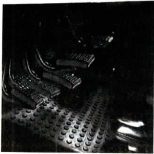
Clutch-operating switches mount on floor and on hand-operated gearshift levers.
