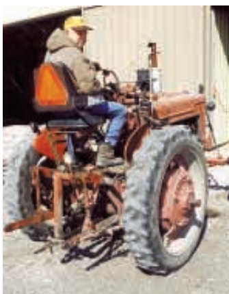
Dunton added a hydraulic pump that's gear-driven off the tractor engine. Pump is used to raise or lower the commercial 3-pt. hitch, which he also added.
