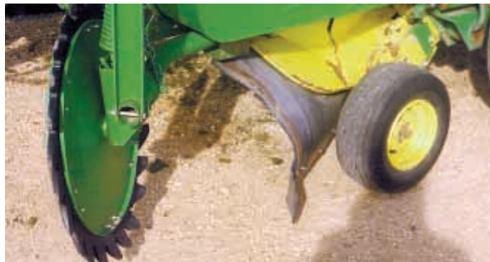
John Hanson made his own scraper blades out of a plastic 55-gal. barrel and mounted them on both sides of the baler pickup.
