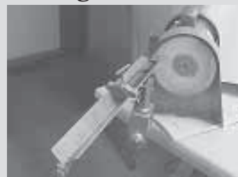
Sharpener attaches to Delta 6-in. grinder with no modification. On other grinders, you may have to drill holes to mount it.
