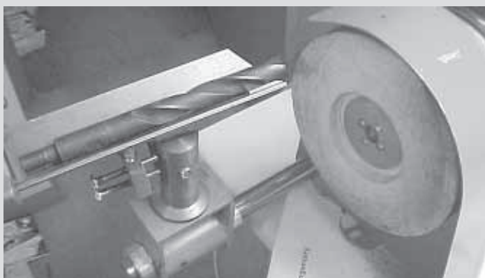
Do-it-yourself sharpener mounts on a 6-in. bench grinder. Handles bits up to 3 in. dia.
