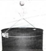
ference of the barrel under the lip and stainless steel brackets prevent any slippage. When the "lift eye" at center is raised by a hoist hook, the cable tightens around the barrel. Works on all barrels 55 gal. and smaller, and can be used on steel, plastic, fiber and open-top drums without damage to drums. Sells for \$55. (John W. Moore, President, Free Enterprise Systems, Inc., P.O.Box 2374, Rapid City, S. Dak. 57709 ph 605 348-5040).
