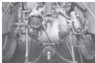
Pulley mounted on pto shaft (left) belt-drives power steering pump. Cylinders connect to tie rods.
