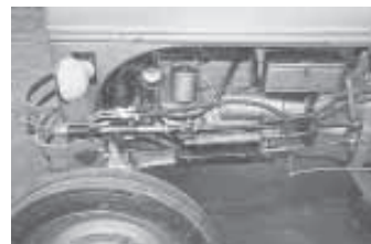
Pulley mounted on pto shaft (left) belt-drives power steering pump. Cylinders connect to tie rods.
