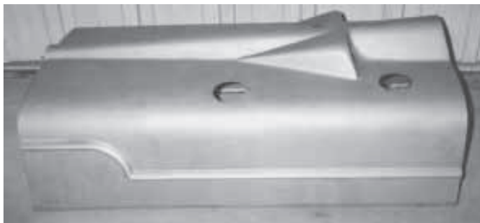
Farmall hood sand-blasted with walnut hull mixture shows no sign of damage.
