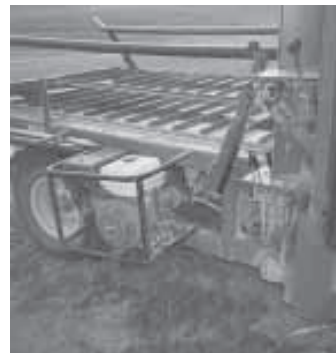
"Continuous drive" self-propelled rig is designed to wrap either round or big square bales without stopping. It can wrap up to 120 big square bales per hour.
