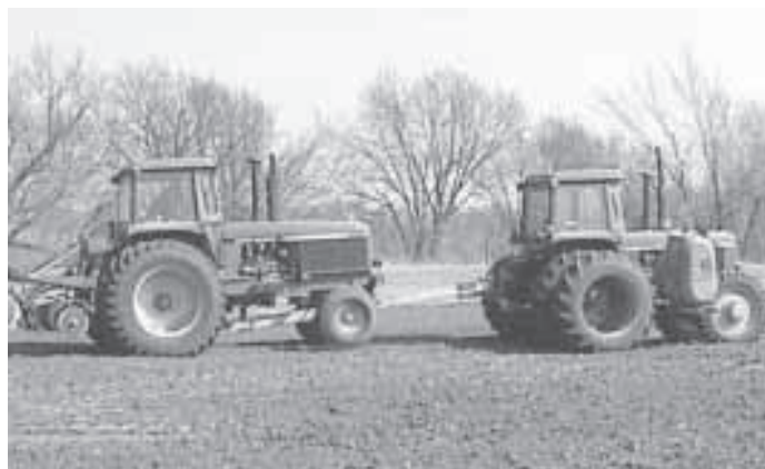
Home-built hitch allows Roy Ferguson to couple two Deere tractors together and drive both at once. He uses the tractors to pull a 15-ft., 3-bar chisel plow.
