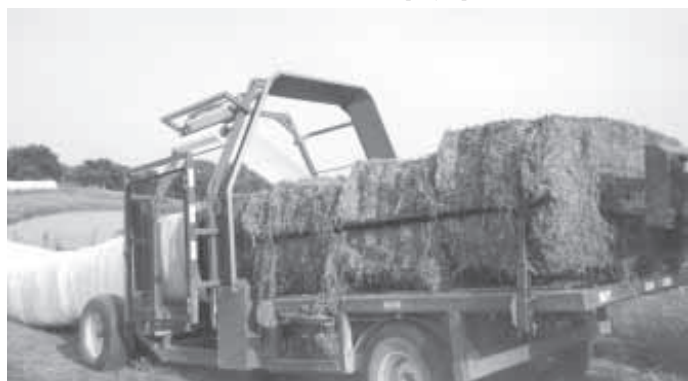
"Continuous drive" self-propelled rig is designed to wrap either round or big square bales without stopping. It can wrap up to 120 big square bales per hour.
