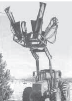
Wedge-shaped spades mount in a square frame that attaches to loader. Makes a hole 32 in. deep and 3 ft. across.
