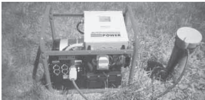
Generator hooks up to an on-off switch, like a float in a water tank. When switch goes to the "on" position, the generator starts up, providing 120 to 240-volt power.
