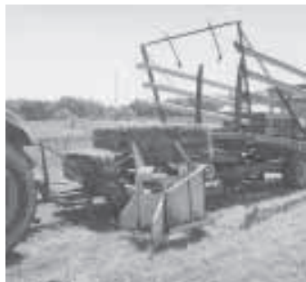
Bales are picked up in the field and then stacked on pallet at back of wagon.
