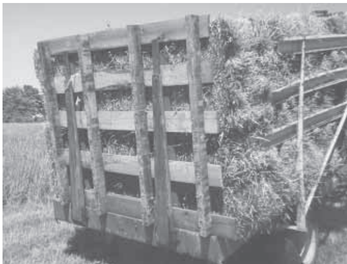
Oversized 5 by 6-ft. wood pallet slips onto wagon's rear forks.
