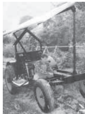
Photovoltaic shade canopy keeps the batteries charged and the operator cool.
