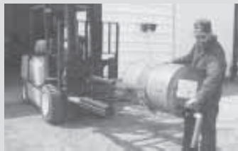
Skid loader-mounted barrel is free to pivot.
