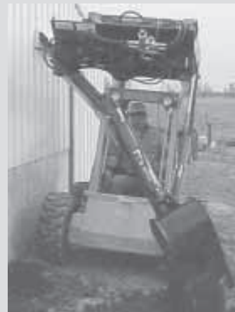
You can dig right alongside foundations with this new skid loader-mounted backhoe, which has a unique pivoting boom.
