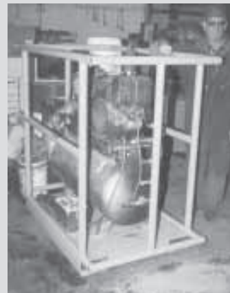
Big compressor and battery mount inside homemade steel cage that's equipped with slots for forklift tines.
