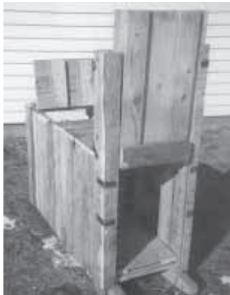
Trap consists of a wood box with a sliding door held up by a rod that’s bumped out of the way when an animal steps on an inclined ramp. Opposite end of trap has a screen-in wall.
