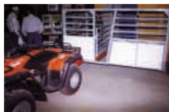
Once calf is inside cage, operator pulls a rope to shut the door.
