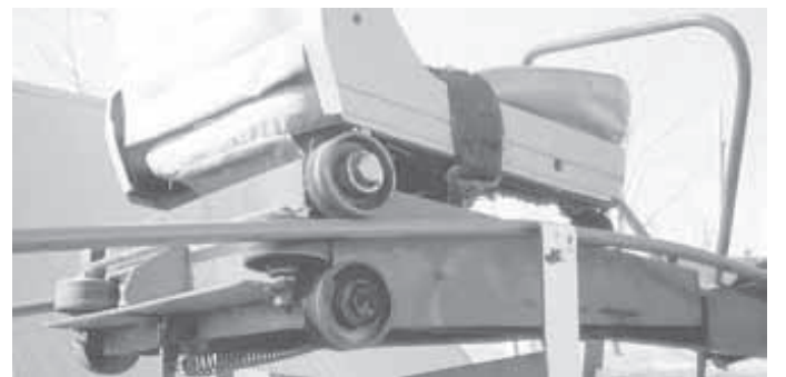
"Coaster car" is equipped with four sets of wheels that ride along a pair of steel rails.
