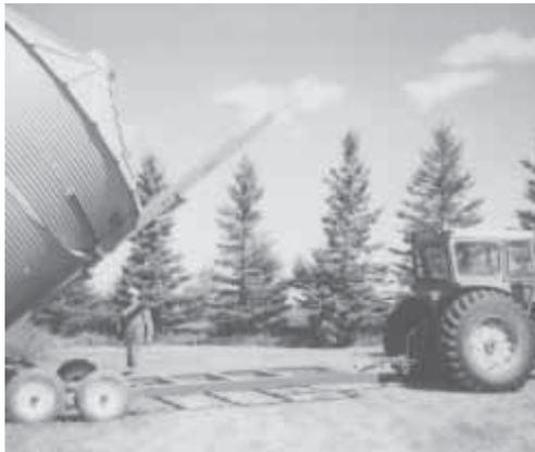
Peter Husak built a hydraulic-operated bin mover that's designed to be pulled by a tractor and rides on two axles. It loads with straps that wrap around bin.
