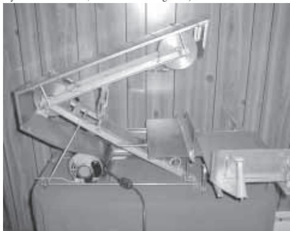
Meat saw is powered by a 1/3-hp, 110-volt electric motor and comes in a 38-in. long box. It snaps together, requiring no tools for assembly.
