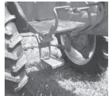
Diamond tread step measures 4 in. wide by 6 in. long. Extended drop model goes about 4 in. lower than standard one.
