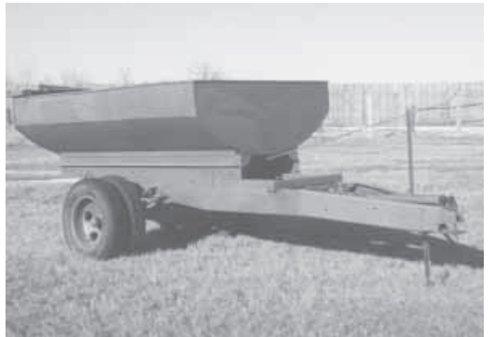
Don and Darrel Hampton used a 10,000-gal. underground gas storage tank and an old truck rear end to make this heavy-duty dump trailer.
