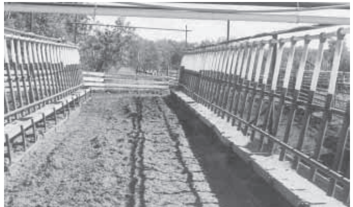
Feed is moved through 190 ft. of 3-in. dia. flexible auger to 40 drop spouts along the length of Babcock's feed trough. Four or five animals can feed from each spout.
