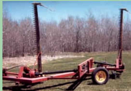
Low-profile frame holds two 9-ft. New Holland sicklebar mowers.
