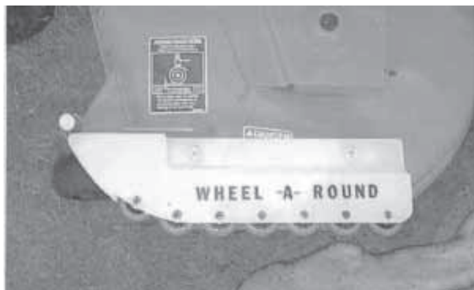
Add-on rollers for decks allow you to get close to trees without doing damage.
