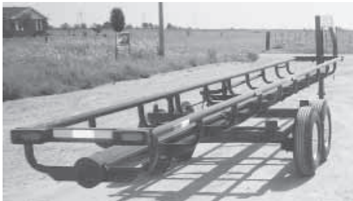
Tandem axle trailer can haul five to eight big round bales at a time.
