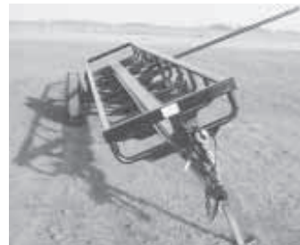
To unload, you pull a lever and trailer pivots to the side.
