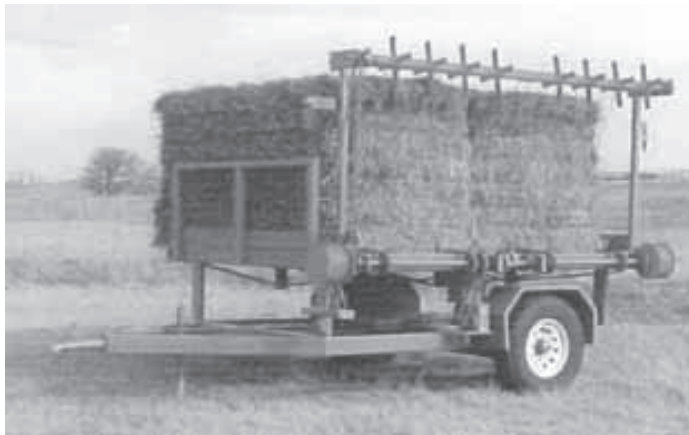
Bale flaker is designed to be pulled by any 1-ton pickup or a tractor and can feed either one or two big square bales at a time.
