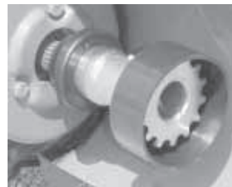
Two-part adapter fits on Deere 9000 series combine's header drive shaft and the driven shaft of the head. No modifications are needed to either head or combine.
