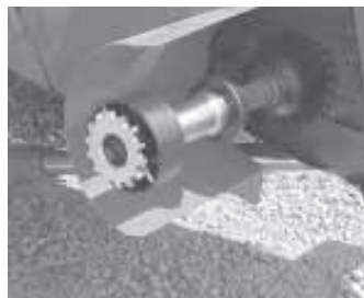
Two-part adapter fits on Deere 9000 series combine's header drive shaft and the driven shaft of the head. No modifications are needed to either head or combine.
