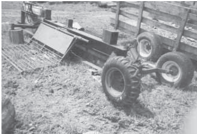
Rear axle pivots to lower big splitting table to the ground. Note that there are two separate splitting wedges.
