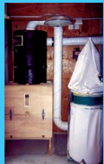
Exhaust system consists of 6-in. dia. PVC pipe and elbows that hook up to a 2 hp, 220-volt vacuum motor.
