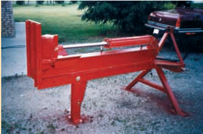
Two-way splitter is powered by a 24-in. cylinder. It can be disconnected from tractor for stand-alone use thanks to legs at either end.
