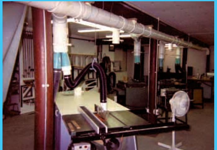
Exhaust system consists of 6-in. dia. PVC pipe and elbows that hook up to a 2 hp, 220-volt vacuum motor.
