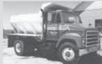
Clair and Warren Wilson mounted the box from a single axle, 2-ton fertilizer spreader truck on their semi tractor.
