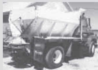
They installed an air-operated pto to drive the belt conveyor and added a 2-in. receiver hitch on back for pulling machinery on the road.
