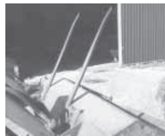
Tines stick up at a 60-degree angle when bucket is level.
