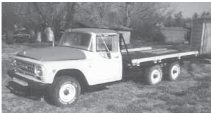
Jerry Ewell converted a 1964 IH 1200 series 3/4-ton, 4-WD pickup into this 6-WD model that's equipped with walking beam rear axles and a 12-ft. long steel flatbed.
