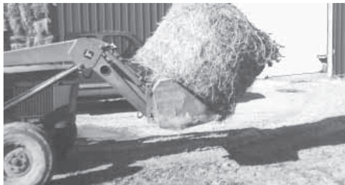
Starr Graham came up with a low-cost bale hauler for his Deere 2240 2-WD tractor by welding a pair of 2 1/2-ft. long steel tines to the back side of the loader bucket.
