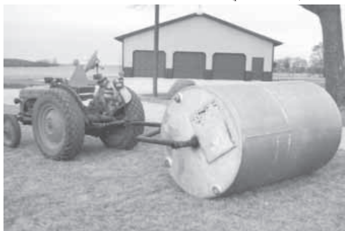
Using mostly scrap materials, Mike Grace built this 7-ft. long, 54-in. dia. yard roller.
