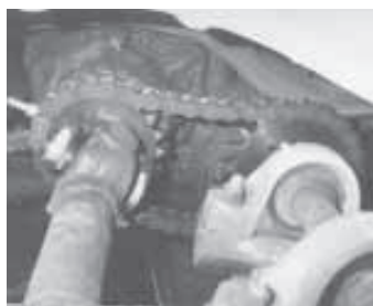
Pickup's original rear end chain-drives the extra rear end that Ewell added.
