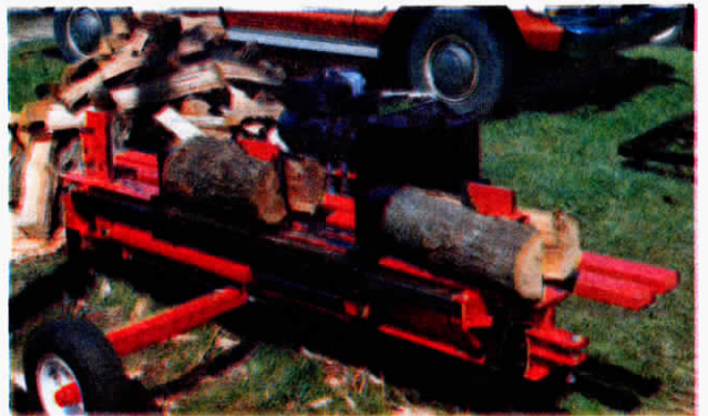
Two-way splitter splits two logs on the forward stroke and two logs on the return.
