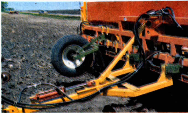
One-way lifting cylinder, above, lifts the converted drill onto lift assist wheels, but floats loosely in the field. Once converted to a trailing type drill, above right, drills can be pulled behind a smaller tractor.
