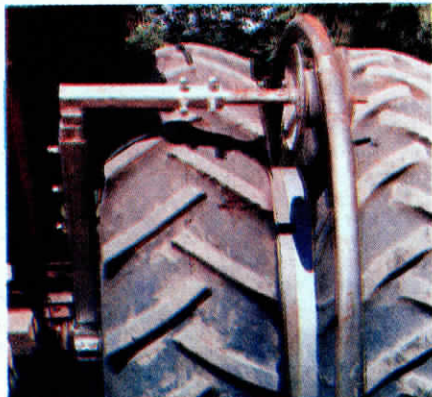
The continuing "chain" of sickle sections can be run clockwise or counter-clockwise. All sections wear evenly.
