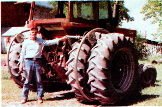
As tractor moves forward, off-center floating ring turns with the wheel to clean out mud (or snow).
